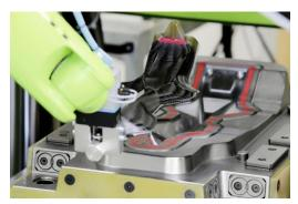
In the composite version, motorcycle number plate holders are 62 percent lighter than purely injection moulded holders. CAVUS technology from KTM enables even complex hollow parts to be mass produced in an automated HP-RTM process. (Pictures: Hennecke)
